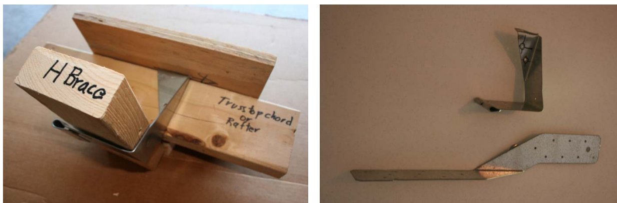
Figure 15.2. On the left the jig is shown support the Horizontal Brace under the rafter. By hitting the jig with a hammer it is wedged between the roof sheathing and the top of the rafter. The left figure shows the jig that was fabricated from a twist strap like the one shown, a Simpson H6 or a USP LFTA6. The wedge part of the jig is about 3/4" long.
