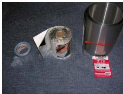
**Some of the materials you can use for temporary patches to holes or tears in metal roofing**
