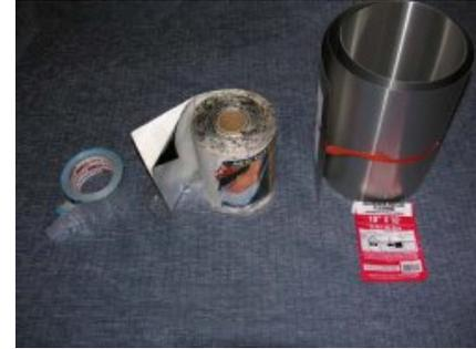
**Some of the materials you can use for temporary patches to holes or tears in metal roofing**
