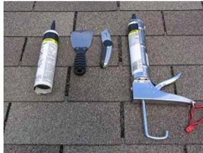
**Tools and supplies needed for temporary patching of holes or to re place torn tabs**
