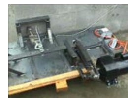
Video: Anchor Pull-Out Test
