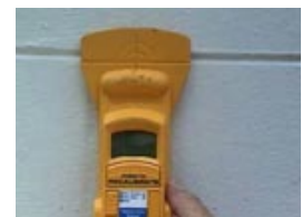
Video: Checking for rebar (click image to view video)
