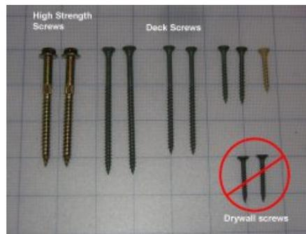
**In any of the structural retrofits, we recommend screws as opposed to nails to avoid nail pops from existing wallboard - never use drywall screws, they are very brittle and will snap off - use the more ductile deck screws or specialty high strength screws.**
